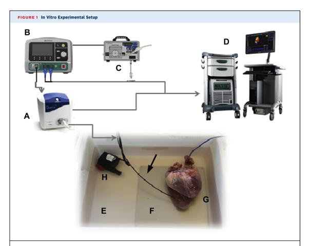
(A) Contact force catheter interface. (B) Ampere RF generator (St. Jude Medical, St. Paul, Minnesota). (C) CoolPoint irrigation pump (St. Jude Medical). (D) NavX electroanatomic mapping system (Endocardial Solutions, St. Jude Medical). (E) Saline bath. (F) Ground platform. (G) Porcine heart. (H) Non-pulsatile pump. (Arrow) TactiCath ablation catheter (St. Jude Medical).
