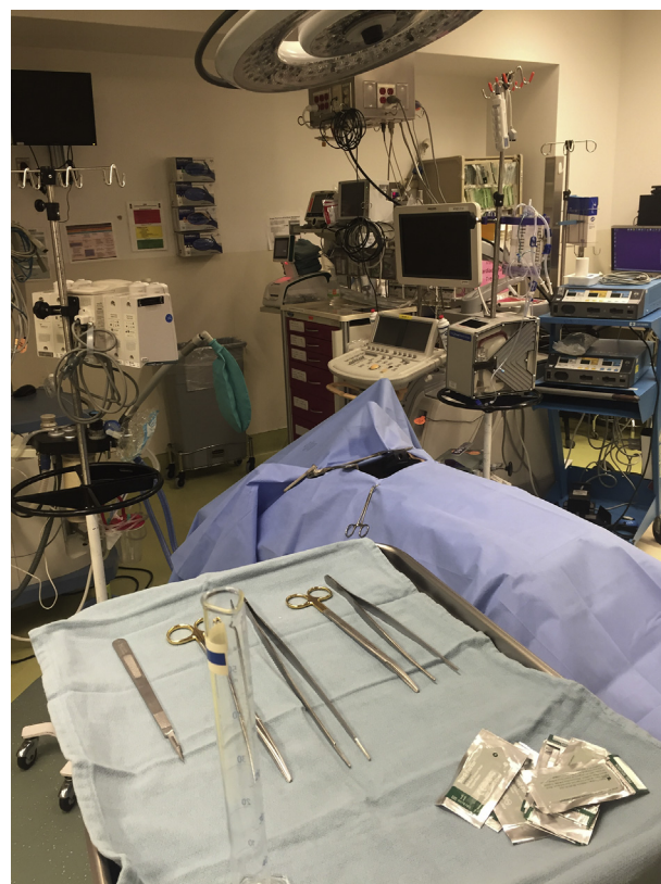
FIGURE 1. Photograph showing the setup of the simulator within an empty operating room. The 3-D print is positioned within a basin placed in the chest cavity of a mannequin. A sternal retractor and drapes help to recreate the field. Basic instruments and the graduated cylinder used to measure resection volumes are shown on the Mayo stand.
