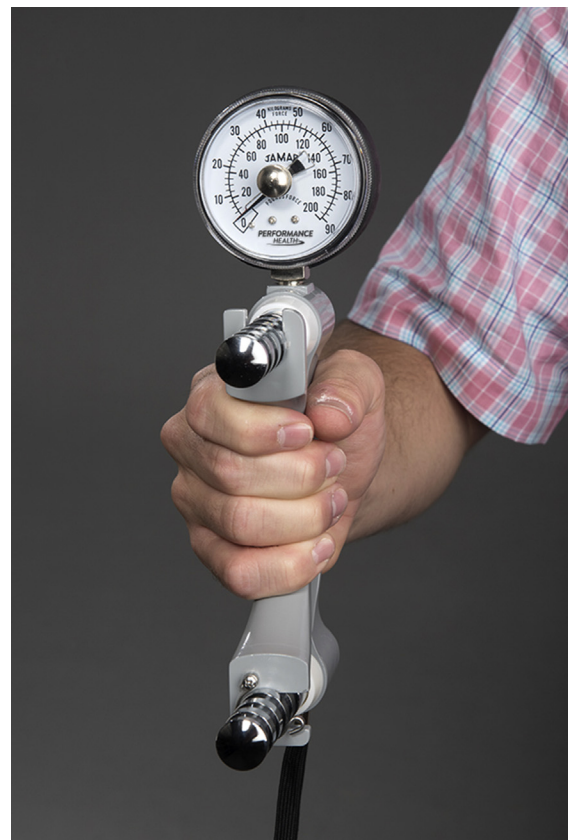
Fig 1. Photograph of calibrated hydraulic hand dynamometer used for grip strength measurement. (Image is reproduced with permission of Performance Health.)
