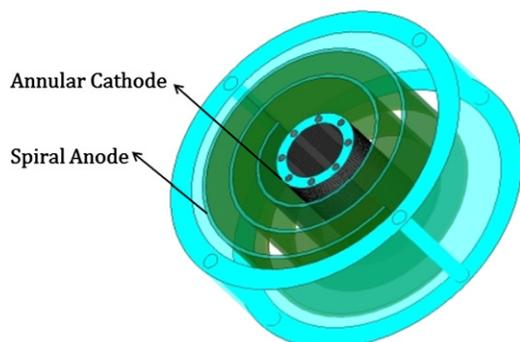
Fig. 1. Schematic diagram of annular single chamber microbial fuel cell (ASCMFC) with spiral anode.
