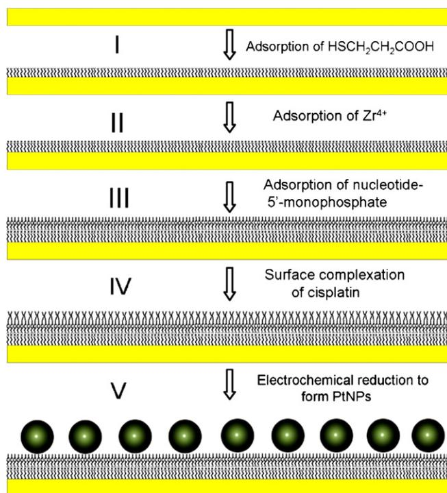
**Scheme 1.** Preparation of nucleotide-5'-monophosphate/ $Zr^{4+}$ /3-mercaptopropionic acid/Au multilayer assembly, binding of cisplatin at the outlayer of nucleobases and electrochemical reducing of cisplatin to form Pt nanoparticles array. Details are in text. Not drawn in real scale.
