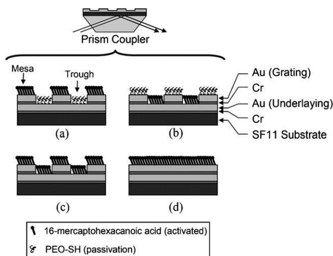
**Fig. 1.** Four biointerface designs (a) binary nano-grating with surface bioreceptors on the nano-grating mesas (b) with surface bioreceptors in the nano-grating troughs (c) uniformly distributed (d) reference surface with planar interface and functionalization.
