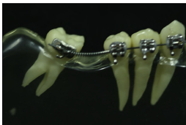
Fig 4. The open-coil spring test specimen.
