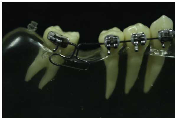
Fig 3. The T-loop spring test specimen.
