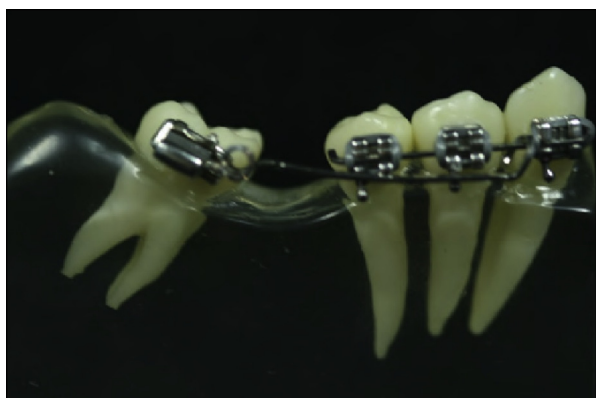
Fig 2. The cantilever spring test specimen.
