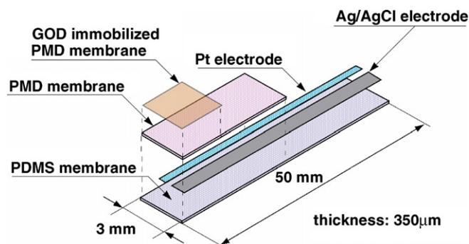
Fig. 1. Schematic structure of the flexible glucose sensor using MPC polymer.
