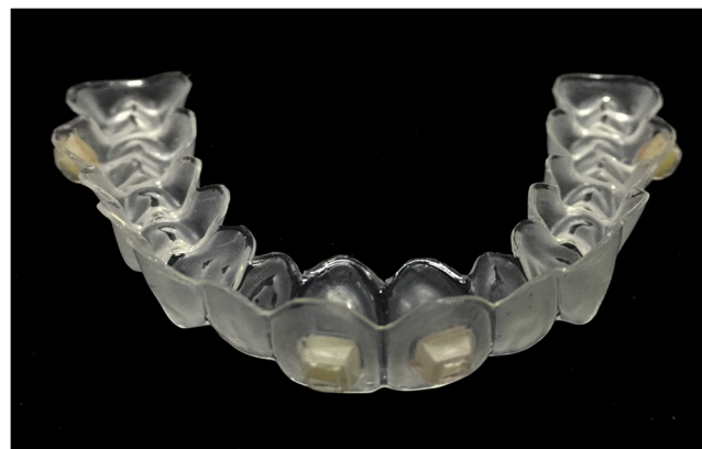
Fig. 1. Intraoral appliances containing 4 specimens. Each niche has 1 opening for acid exposure, and the specimen was fixed 0.5 mm beneath the appliance surface to prevent abrasion from the tongue and oral mucosa.
