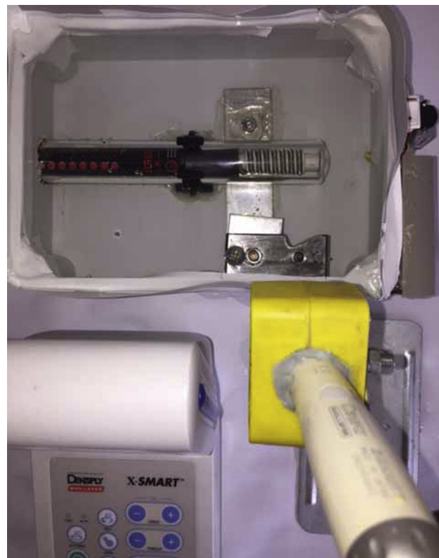
Figure 1. The experimental setup of the cyclic fatigue test device for the simulation of the intracanal temperature.
