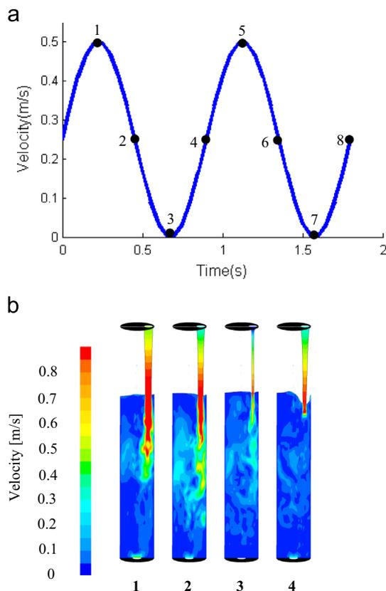
**Fig. 1.** (a) Inlet velocity of the airtrap for two cycles. (b) Instantaneous velocity profile of a middle plane in the blood flow in the venous airtrap at different stages.
