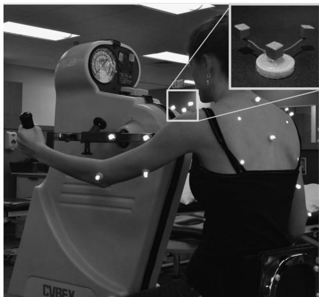
Fig. 1. Cycle setup with markers and acromion marker cluster.
