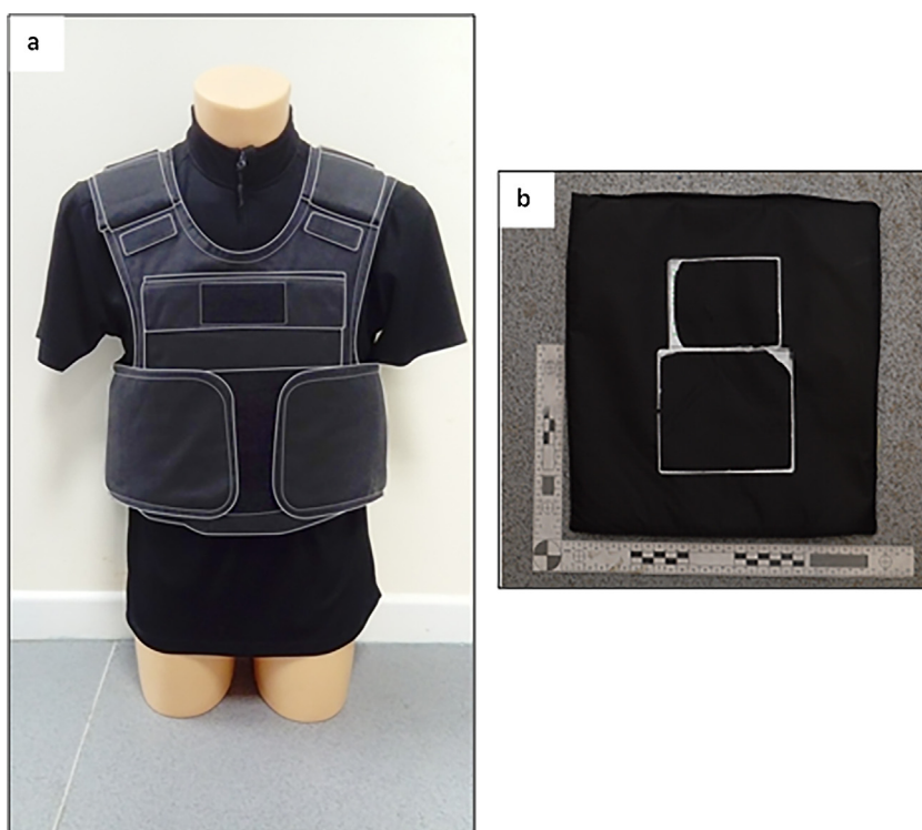
Fig. 1. a) Typical police polo shirt with carrier vest over the top and b) standard UK ballistic test panel of HG1/A + KR1 body armour.
