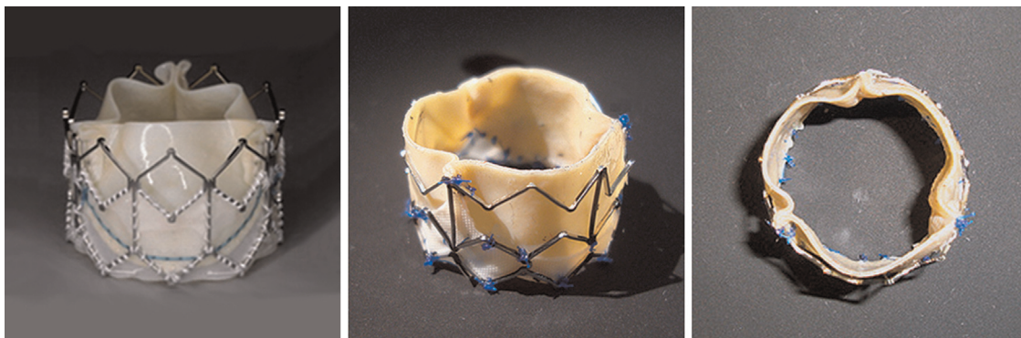
Fig. 1. (Left) Edwards SAPIEN XT valve. (Center and right) Side and top view of homemade 23 mm transcatheter aortic valve; leaflet geometry was based on the SAPIEN XT valve design.
