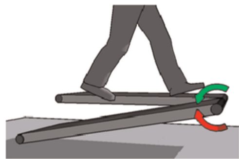
Fig. 2. One single split-belt is lowered to apply the vertical perturbation at mid-stance of the right leg. The green arrow illustrates the rotation of the split-belt downwards during the drop of the walking surface and the red arrow illustrates the return of the walking surface upwards, back to horizontal level. (For interpretation of the references to color in this figure legend, the reader is referred to the web version of this article.)
