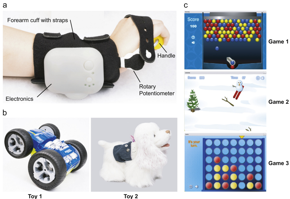
Fig. 1. Controller, remote controlled toys, and computer games. (a) Specially designed play controller used to wirelessly control toys and games. A potentiometer in-line with the flexion–extension axis records wrist motion. Wrist position thresholds to trigger play are set using buttons on the electronics case. (b) Remote controlled toys: BounceBack Racer ® (Toy 1) and GoGo ® (Toy 2). (c) Computer games: Bouncing Balls ® (Game 1), Snowman ® (Game 2), and Lineup ® (Game 3).
