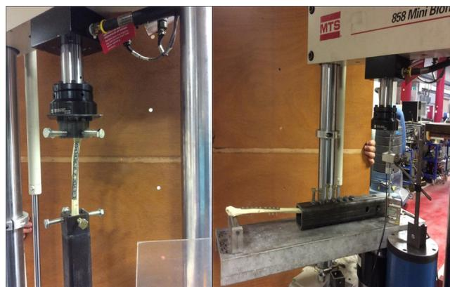
Fig. 1. MTS 858 Mini Bionix rig with sawbone construct for torsion testing (left) and lateral bending (right).
