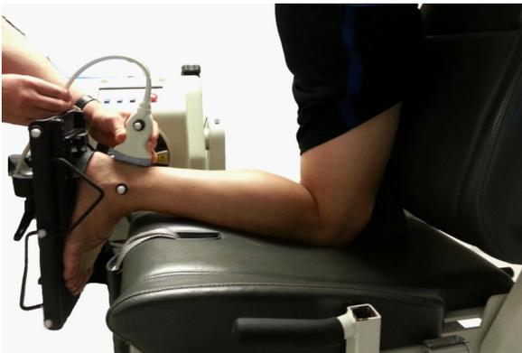
**Fig. 1.** The setup for the collection of moment arm data. This is the same setup for the collection of the brightness and stress data with a change in probe position and/or orientation. Note the ankle and knee at  $90^\circ$  and markers placed on the malleoli and at the center of the ultrasound transducer.
