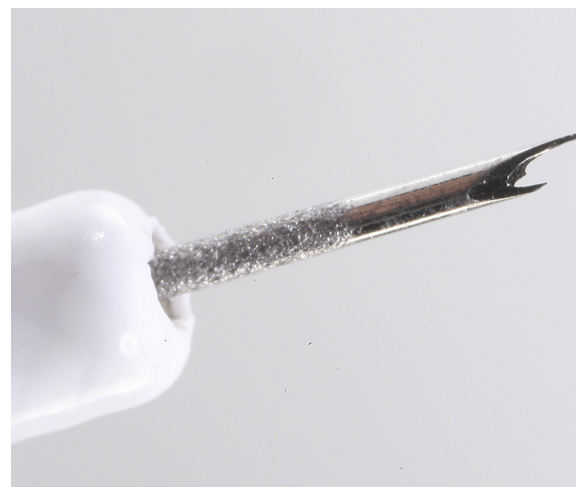
Fig. 1. The tip design of the newly developed SharkCore™ EUS-FNB needle, featuring a multifaceted opposing bevel incorporating two sharp points and 6 cutting-edge surfaces, intended to promote tissue capture with maintenance of its architecture; reproduced with the permission of Medtronic.
