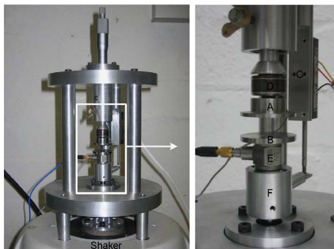
Fig. 1. Custom built high speed cyclic testing rig. (A) Top platen; (B) bottom platen; (C) LVDT transducer; (D) static load cell; (E) dynamic load cell; and (F) connection with shaker.
