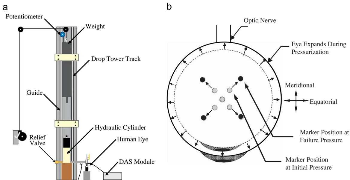
**Fig. 1.** Schematic representation of high-rate pressurization system (left) used to determine material properties and the expansion of a human eye shown with optical markers (right).
