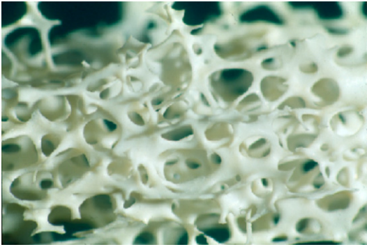
Fig. 1. At the microscale, cancellous bone is a heterogeneous composite material formed of trabeculae and bone marrow. Photograph of trabecular bone is courtesy of Scott C. Miller.
