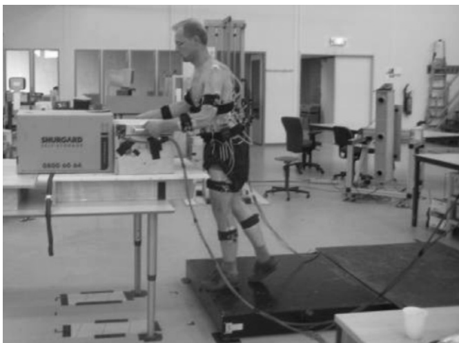
Fig. 1. Experiment setup for the lifting tasks. Marker clusters were used to monitor the movement of body segments.
