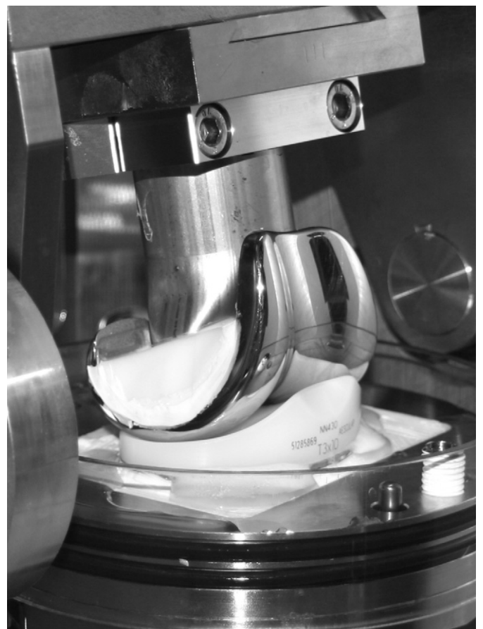
Fig. 3. The ultracongruent fixed bearing TKR implant used in the study (mounted in a wear station of the simulator).
