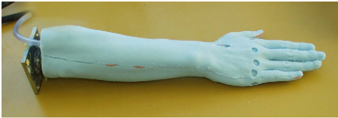
Fig. 1. The hand and forearm model. Note: the surface of the hand had 12 concavities where internally wired pressure sensors were embedded (10 mm diameter and 3 mm thickness). The pressure data was not reported in the present study.
