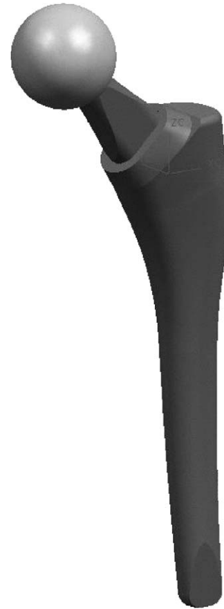
Fig. 1. Solid model of the AncaFit anatomical stem assembled with a 28-mm ball-head and a straight modular neck.
