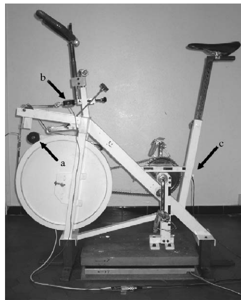
Fig. 1. The cycle ergometer mounted on the force platform for 3D pedal force measurement. The bicycle was equipped with a displacement transducer (a), a force transducer (b) and position transducer (c).
