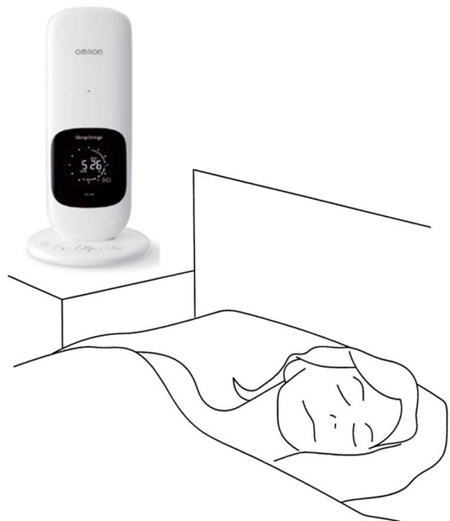
Fig. 1. The original snore detection device was equipped with a microphone to record the snores and an algorithm to evaluate snoring apart from outside noises. The device was set with approximate dimensions and placed relative to the bed and the snorer.
