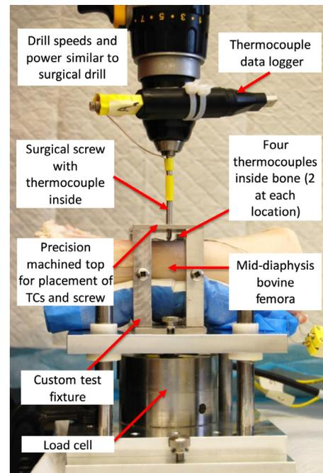
**Fig. 2.** A custom fixture was used for recording temperatures while inserting external fixation screws.
