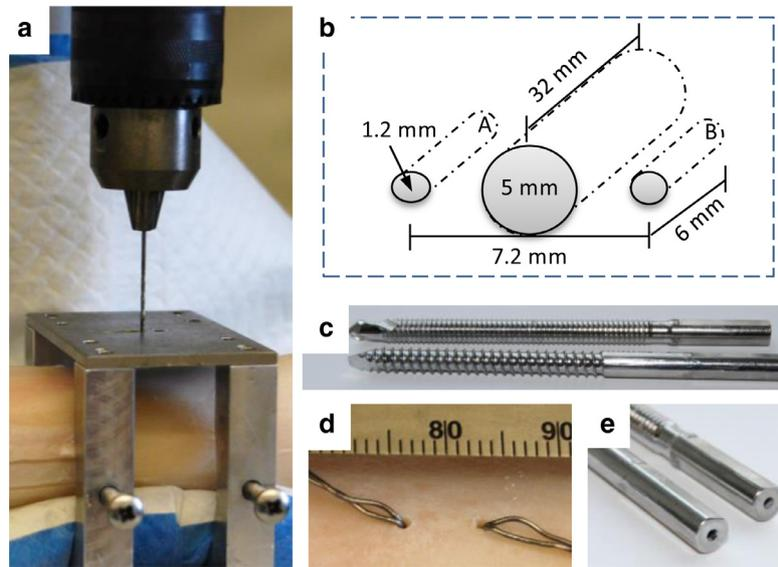
**Fig. 1.** (a) A custom test fixture with a machined template was used on a drill press for the thermocouple holes in the bone. (b) The spacing of the thermocouple holes placed them 0.5 mm from the outer edge of the center screw hole. (c) Standard Schanz screws and self-drilling tip Schanz screws were cut down in length for placement of a thermocouple inside each screw. (d) Two thermocouples were placed in each hole inside the bone. (e) One thermocouple was placed inside each screw for testing.
