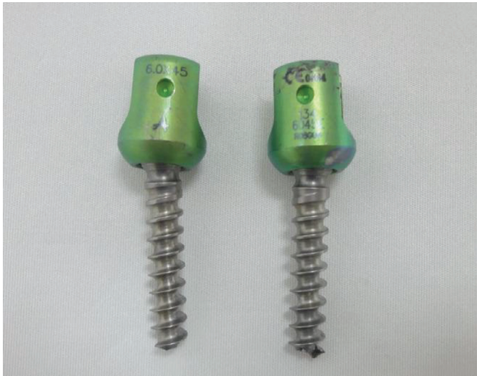
Fig. 1. Ruptured cannulated screws with nine radial holes located in the distal one-third of the screw shaft (SmartLoc Evolution System: Cannulated Screw, 60 mm × 40 mm, A-Spine, Taipei, Taiwan).
