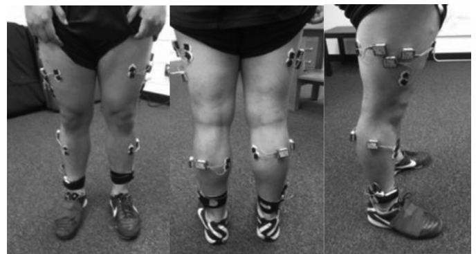
Fig. 1. Anterior, posterior and lateral views of EMG electrode setup.
