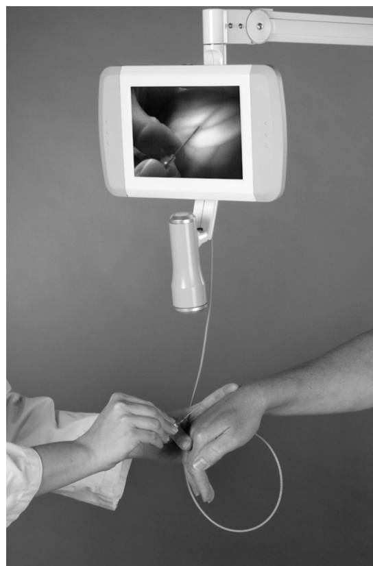
Fig. 2. Close-up of the display and camera in use. The display and the puncture site are at the same distance to the eye of the user. The puncture site is shown approximately life-sized on the display.
