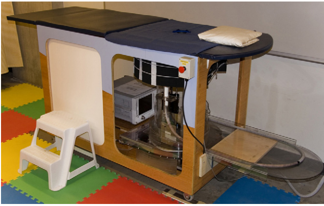
Fig. 1. The TSAR system prototype. The breast extends through the hole in the table top. A tank under the table (covered in black material) contains canola oil and the sensors of interest.
