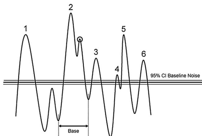
**Fig. 1.** Surface electromyographic (sEMG) interference pattern to illustrate the difference between a spike and a peak. A spike is composed of a single upward and downward deflection that are greater than the 95% confidence (CI) interval for baseline activity. There are six spikes and spike #2 one peak (circled).
