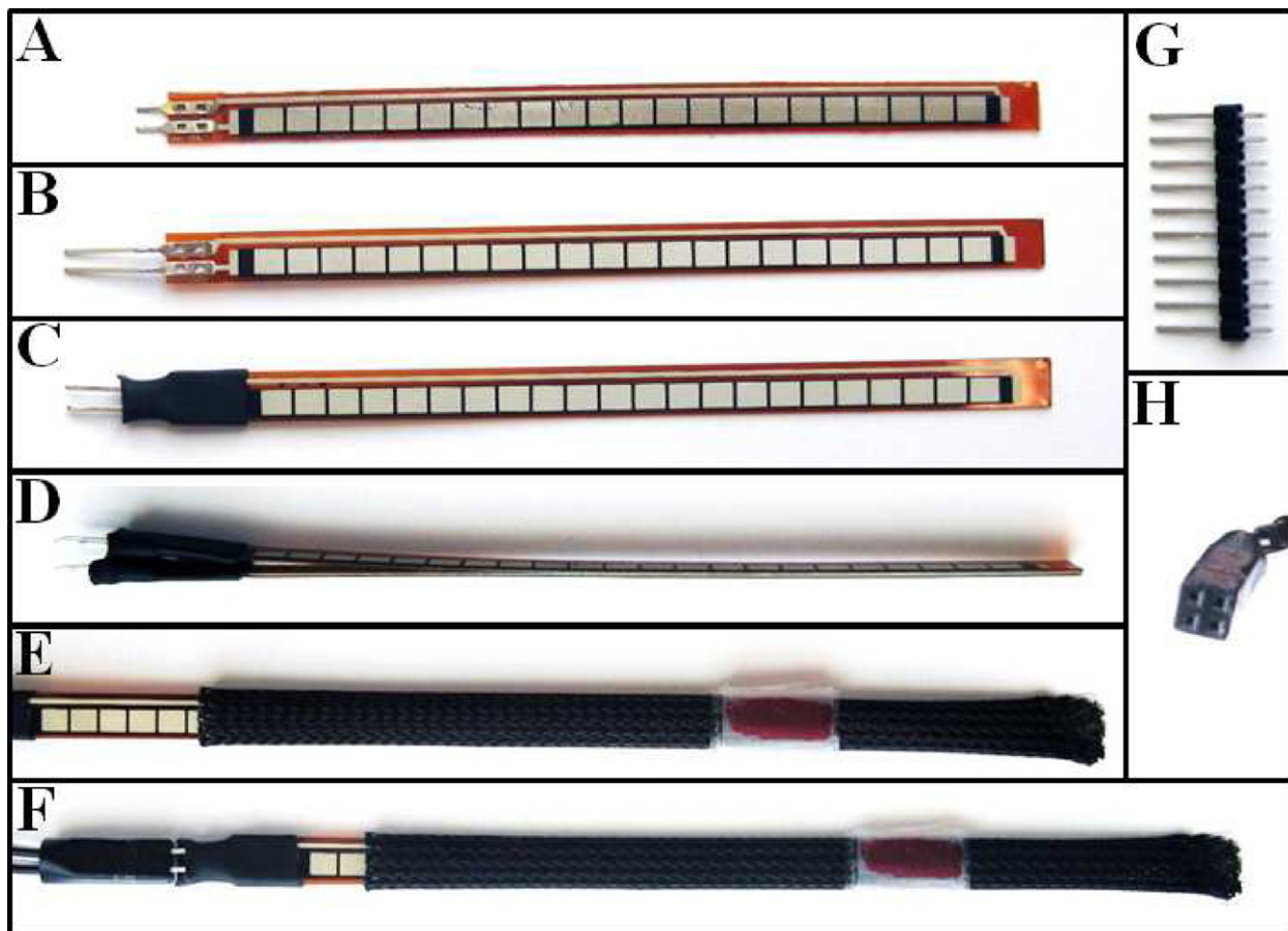
Fig. 1. (A) A 6.35 mm × 114.3 mm flex sensor before any modification (Spectra Symbol, Salt Lake City, UT), (B) with soldered male header pins (made from G), (C) with heat-shrink tubing for insulation. (D) Two flex sensors placed back-to-back, inserted into (E) expandable PET sleeving to enclose all electrical components (shown partially inserted). (F) Final goniometer assembly was plugged into (H) female headers. Sleeving was taped to female headers with duct tape to strengthen physical stability. The other end of sleeving was burned closed with fire. A plastic conduit made from transparency film was slid onto the sleeving to facilitate low-friction movement during use.
