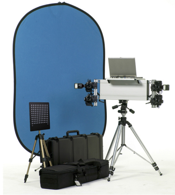
Fig. 1. The Di3D stereophotogrammetry system including, dual pod head, blue screen background, calibration target and carrying cases.
