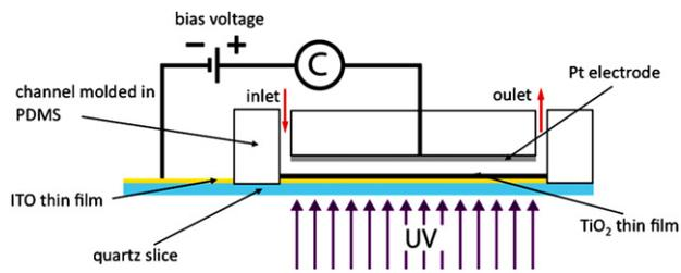
**Fig. 1.** Schematic representation of the photocatalytic cell system. A PDMS microchannel, where liquid flows through input and output ports, is bonded on a pretreated quartz slice. An ITO/TiO<sub>2</sub> junction is in fact deposited on the quartz surface. The top wall of the channel is covered by a Pt electrode, connected directly to the ITO layer, thus closing an electrical circuit.
