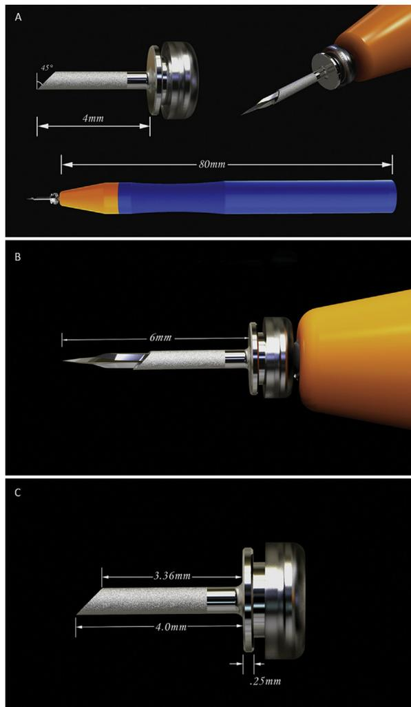
**Figure 1.** The trocar-anterior chamber maintainer. *A:* Cannula, bevel, and handle. *B:* Trocar blade. *C:* Cannula bevel.
