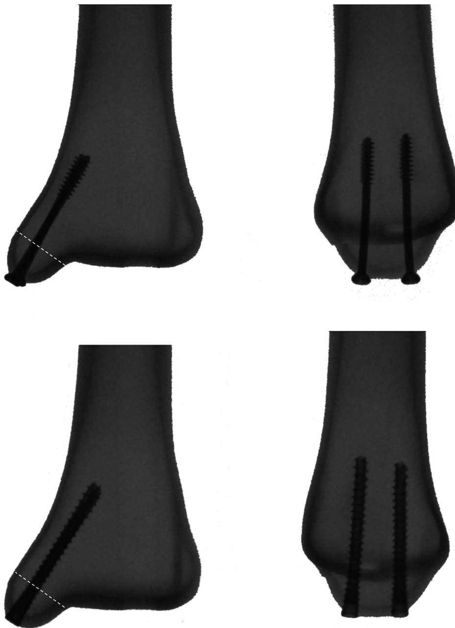
Fig. 1. Representative anterior-to-posterior (left) and lateral (right) X-rays of the parallel unicortical (top) and headless compression screw (bottom) constructs. Dashed lines indicate osteotomy cuts.
