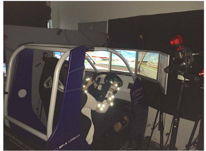
Fig. 1. Study participant performing the formal driving simulation in an OptiTrack™ motion tracking system. The study participant is seen wearing OptiTrack™ motion trackers and seated in the MUARC portable driving simulator. OptiTrack™ cameras can be visualized at various vantage points.
