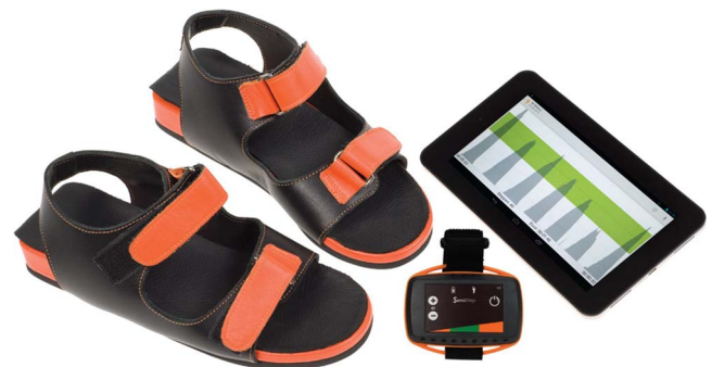
Fig. 1. The different parts of the SensiStep system [19]. The force sensor was placed inside the sole of the custom-made sandals. Real-time, visual biofeedback was shown to both the participant and the healthcare professional via the tablet as a green bar (i.e. target weight) and grey step curves (actual weight). (For interpretation of the references to colour in this figure legend, the reader is referred to the web version of this article.)
