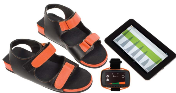
Fig. 1. The SensiStep system. Real-time visual biofeedback was shown on the tablet as a green bar (i.e. target weight) with grey step curves (actual weight). Both the participant and the physical therapist had insight in weight bearing during the feedback session. (For interpretation of the references to colour in this figure legend, the reader is referred to the web version of this article.)
