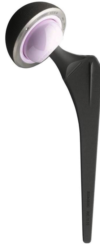
Fig. 1. A hemispheric titanium alloy cup with plasma-sprayed coating (Bencox; Corentec, Cheon-An, Korea) and a grit-blasted, tapered, double-wedged, titanium alloy stem (Bencox; Corentec) with a fourth-generation ceramic-on-ceramic bearing (BIOLOX Delta; CeramTec, Plochingen, Germany).
