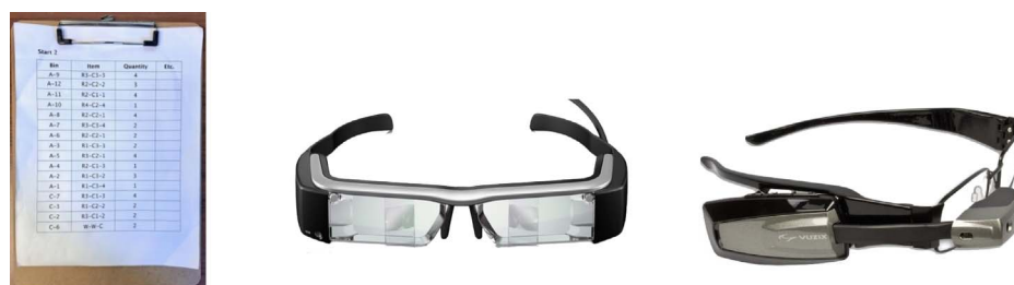
Fig. 1. Technology types: paper list (Left; text font size = 18 pt.), commercially available binocular (Middle; Epson Moverio BT-200), and monocular head-worn display (HWD) (Right; Vuzix M100).
