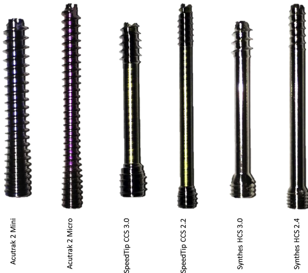
FIGURE 1: The 3 headless compression screw designs studied (left to right): Acutrak 2 Mini and Micro, Medartis SpeedTip CCS 3.0 and 2.2, and Synthes HCS 3.0 and 2.4.
