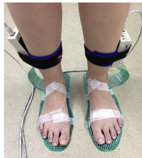
Fig. 1. Sensor placement for the foot. A sensor sheet was taped to the bare sole of all subjects. A lightweight transducer unit was strapped to their legs. A cable was used to connect the transducer to the computer. After calibration, all subjects walked along an even floor at their usual speed. Recordings were made at 50 Hz for 5 s. Data were collected from a mean of 3.3 consecutive steps (3–4 steps).
