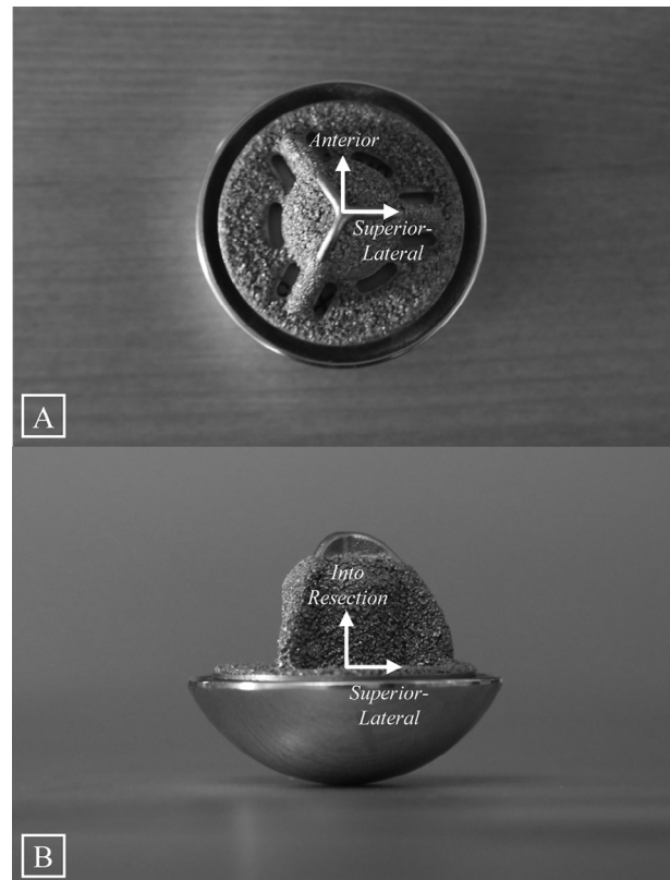
Figure 2 As an example, the Tornier Simpliciti implant is presented to demonstrate that a stemless implant-relevant Cartesian coordinate system should be constructed with axes directed (A) superior-laterally, anteriorly, and (B) perpendicular to the underside of the implant.
