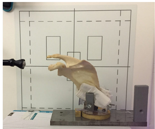
Figure 1 Holding device allowing incremental rotation of the bone around both the horizontal and vertical axes. The scapular body was centered on the digital radiograph receiver.
