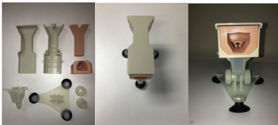
Fig. 1. Views of laryngeal surgical simulation model assembled and disassembled. Legend: Left-Disassembled; Middle-Assembled Top View; Right-Assembled Inside View.
