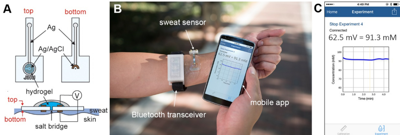
Fig. 1. Wearable sweat sensor and mobile app. (A) Schematic illustration of the sweat chloride sensor. (B) Sweat sensor with integrated salt bridge, Bluetooth wireless transceiver, and mobile application on a smart phone. (C) Captured image of the mobile application during a sweat test.
